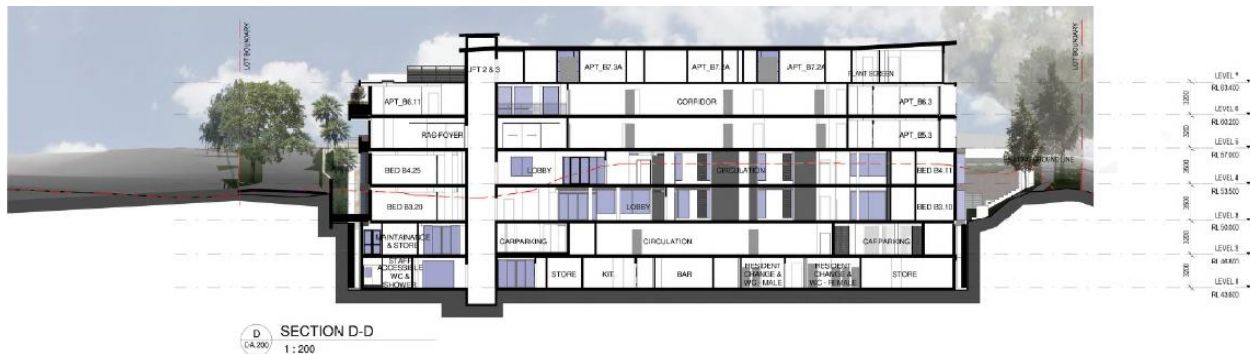
Figure 15: Indicative north-south section of proposed scheme (source: Thomson Adsett).
